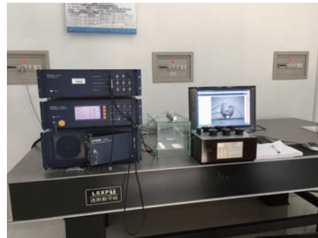
图12 变幅杆共振频率及位移分布的实验测试装置图 Fig. 12 Experimental set-up for the frequency and displacement distribution measurement of the ultrasonic horn
