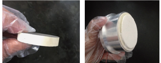
(a) 1-3型压电复合材料样品
